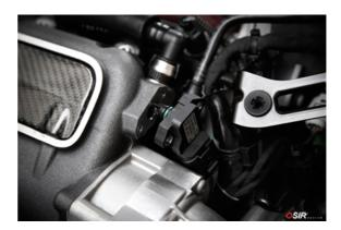
1. Locate and remove the MAP sensor on the intake manifold.
