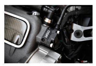
Lubricate the O-Ring on the O-TAP B body with engine oil and secure both sensor and the O-TAP B into the intake manifold with the supplied long screws.
